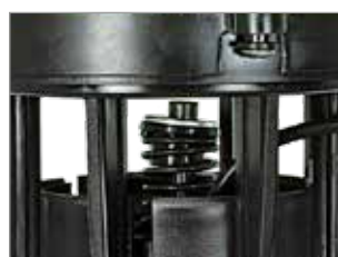
ELECTRICAL FILTER SHAKER
